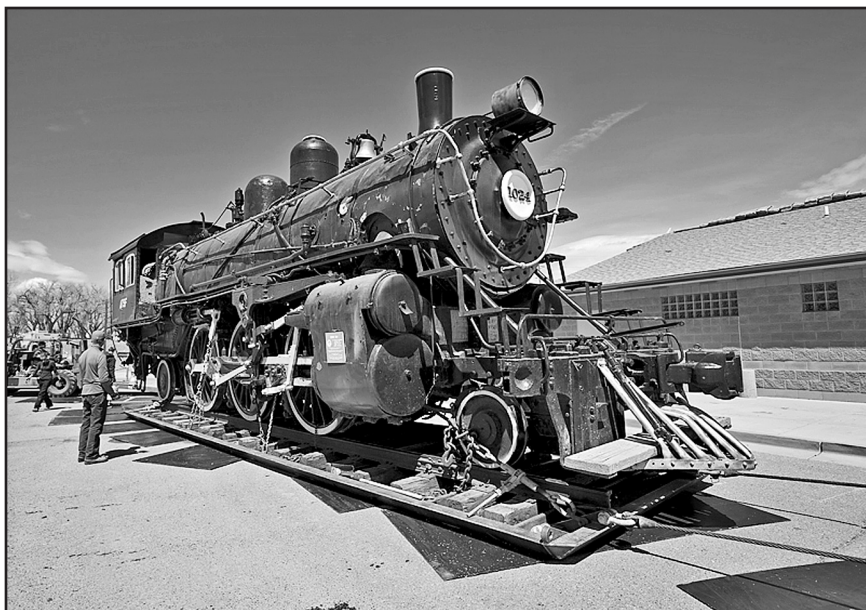
Santa Fe Steam Locomotive #1024 on the custom-fabricated steel pan with a section of panel track. – Photo © 2013 Roger Hogan.
